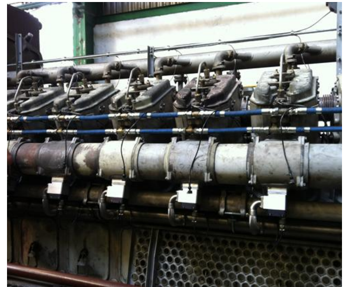
Scheme of gas injectors on engine (left) and picture (right)
