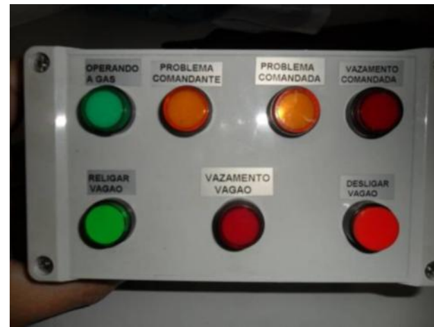
Tender car panel inside locomotives cabin
